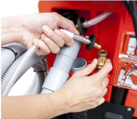
12. Disconnect the grey hose by pulling the hose up and out and connect the grey hose on the Upholstery hand tool to the machine.
