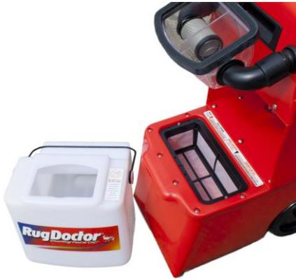
2. A) Fill the lower red tank (underneath the recovery tank) with 9L of hot tap water and 2/3 cup of Rug Doctor cleaning solution. Ensure that the cleaning solution and hot water does not exceed above halfway up the filter.
